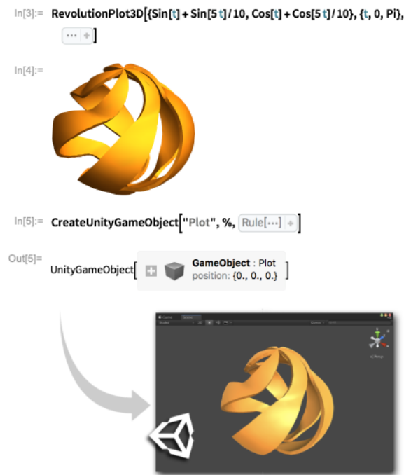
Figure 2.6: Plots, graphics, and geometric objects are automatically converted to Unity's mesh format during the creation of a game object. 26
